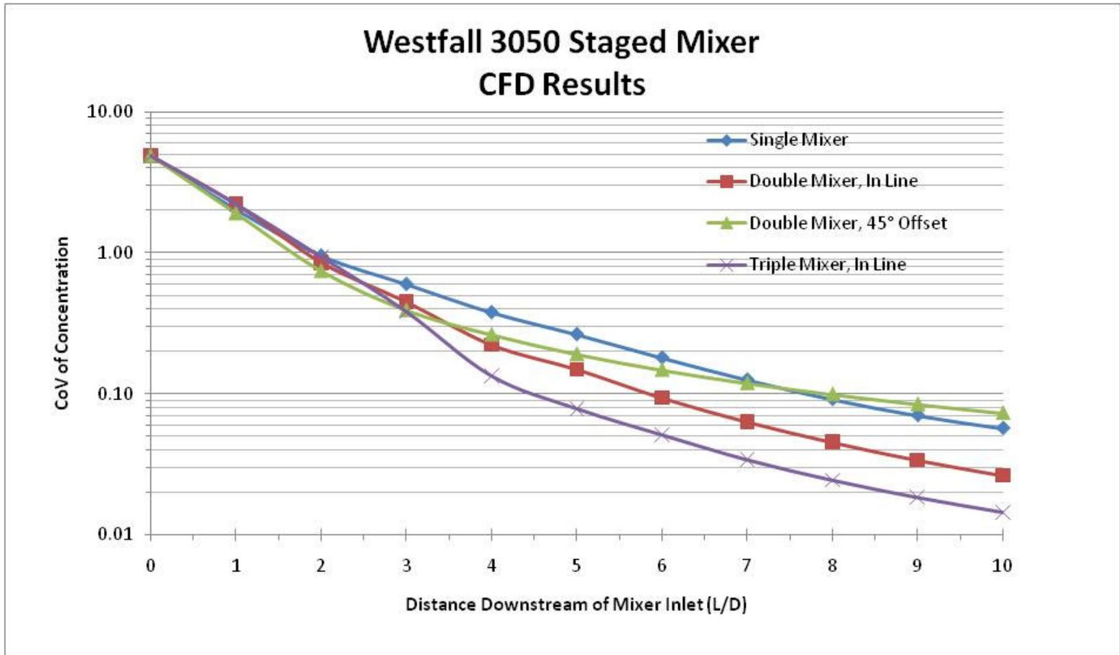
CoV of Concentration in a 6-in ID steel pipe with 2 opposing injection ports, and a mixed tracer concentration of 2%.
